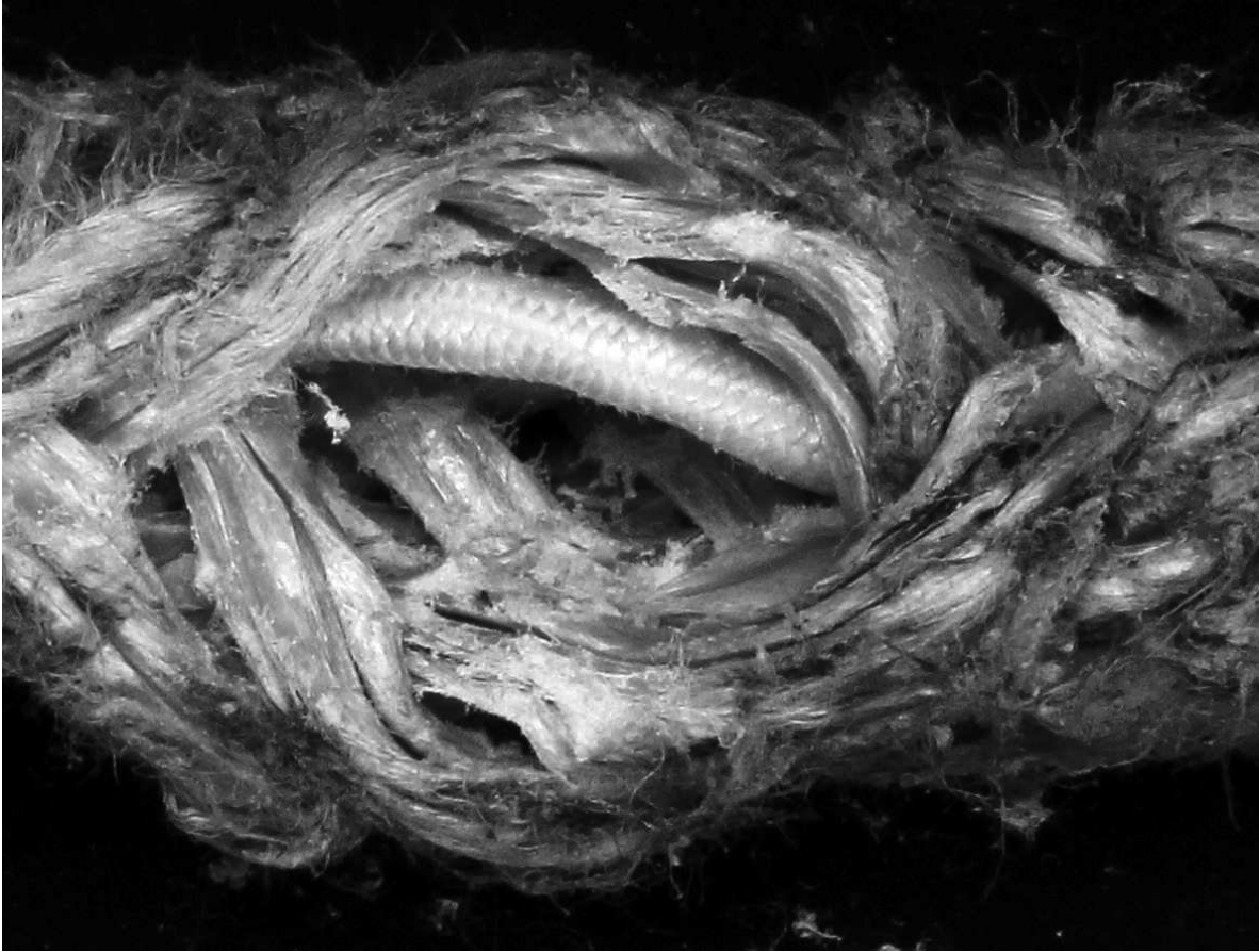
Figure 30-2.8.2-3 Damage Inside the Rope
