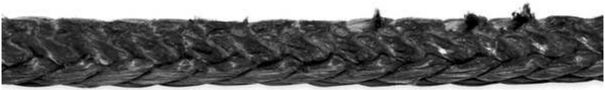
Figure 30-2.8.2-5 Melt Damage Due to Heat
