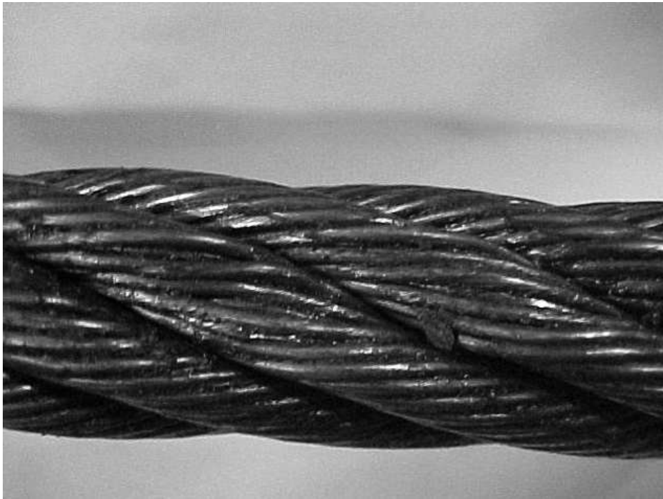
Figure 30-1.8.2-5 Distortion of Rope Structure — Crushing
