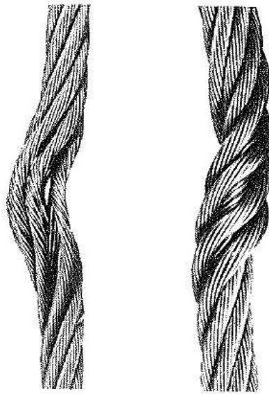
Figure 30-1.8.2-2 Distortion of Rope Structure — Kink
