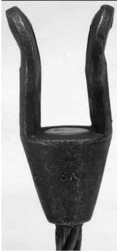
Figure 30-1.8.2-10 Damaged End Terminations
