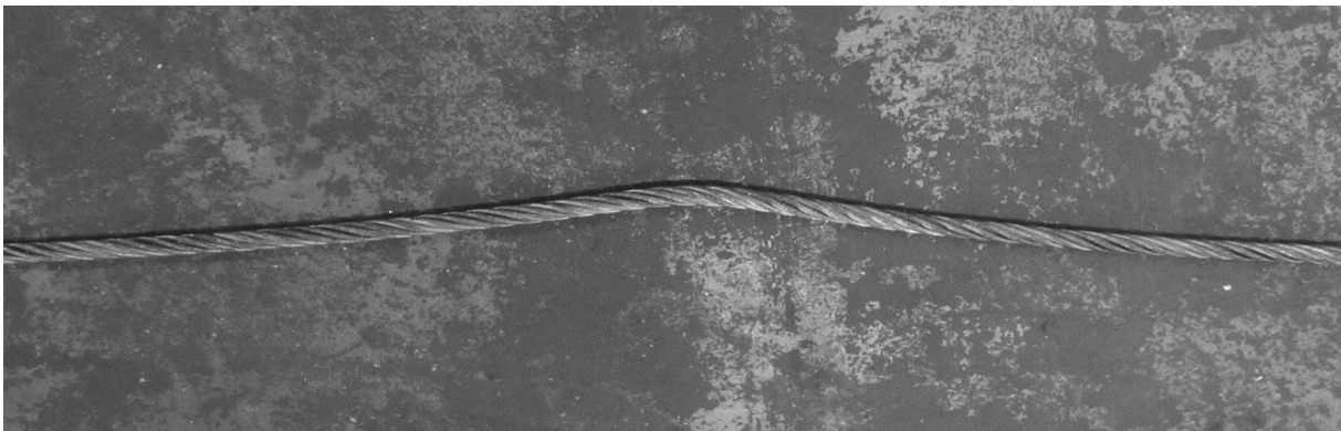
Figure 30-1.8.2-3 Distortion of Rope Structure — Dogleg
